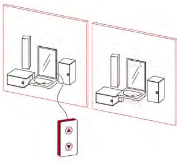
**The patented-system Goman integrate** the mirror-block furniture with a mechanism for wash basin support, electrically movable, for the lifting/lowering action of the block system (mirror and wash basin). This will allow achieving the ideal level, which follow the specific norms to its use by the users (disables, old people, or children).
